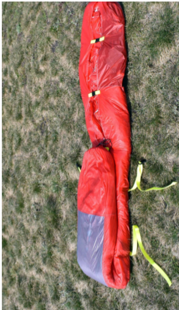
Step 5 Fold the wing in the first 1/3 part starting from the trailing edge
