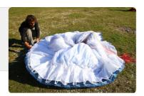
**Step 2.** Group LE reinforcements with the A tabs aligned, make sure the plastic reinforcements lay side by side.
