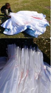
**Step 4.** Group together the middle/trailing edge of the wing by sorting the folds near the B, C and D tabs.
