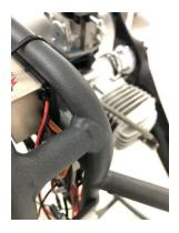
Before any flight, perform a complete inspection of the frame, looking for any evidence, like fractures on the paint surface, that could hide fractures on the welded connections.
