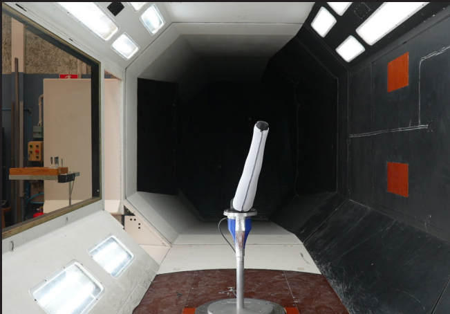
Figure 5.a Seam in usual position, exposed to the incident wind.
