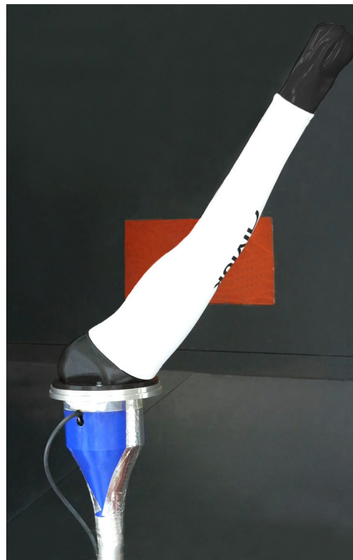
Figure 3. Accelerated flight position tested with R-Series Speedarms fabric.
